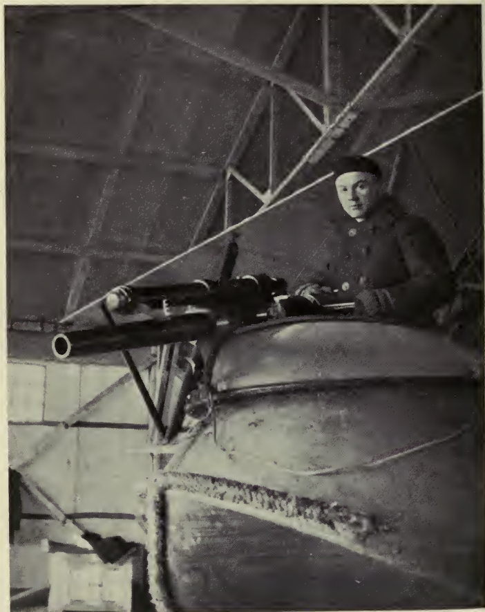
(C) Kadel & Herbert Gun Mounted on the Carriage of American Dirigible Used for Destroying Submarines
